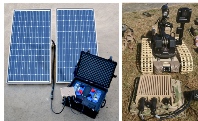
The SPACES power module charging 24 V lead-acid battery array using power from 220W rigid solar panels and SPACES power module stacked with foldable solar panel.
